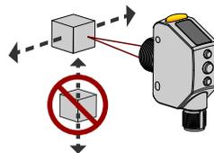
See the following figures for examples of correct and incorrect sensor-to-target orientation as certain placements may pose problems for sensing some targets. The Q4X can be used in the less preferred orientation and provide reliable detection performance; refer to the *Performance Curves* for the minimum object separation distance required for each case.
