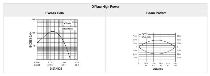
Convergent mode performance curves are based on a 90% reflectance white test card.
